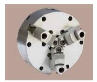
SELF-CENTERING GUARANTEED TO 0.0005" STOCK NO. 1057-0008 FEATURES: TWO-PIECE REVERSIBLE JAWS HIGH STRENGTH SEMI-STEEL BODY LATHE CHUCK RUNOUT ADJUSTABLE TO .0005" BY 4 SIDE SCREWS ALL JAWS ARE STANDARD AMERCIAN TONGUE ANG GROOVE CHUCK DIAMETER 8..15" THRU HOLE 2.48" MAXIMUM GRIP 7.30" WEIGHT 35 lbs.
