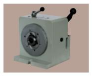
1027-0125(F43125D) can be mounted on milling machine, grinding machine, drilling machine and other machine tools. It is Designed for using and indexing in both horizontal and vertical position and can carry out 2,3,4,6,8,12,24 divisions. This product is equipped with a face plate or chuck.
