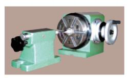
1026(F58) manually operated indexer, which cac be mounted either vertically or horizontally, is mainly used on milling and boring machines. With non-lifting Hirth couping indexing, it features high accuracy and perfect rigidity.
