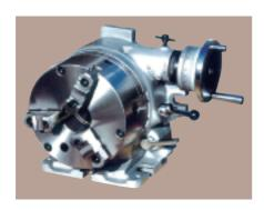
Type 1025 (F3) super spacer is designed for using and indexing in both horizontal and vertical position.it is the most optimum in use for milling machines, grinding machines, drilling machines planer etc. The divisions in 2, 3, 4, 6, 8, 12, 24 are permitted by notched plate, any desired angular indexing can be performed by worm shaft, two methods can be switched over conveniently.
