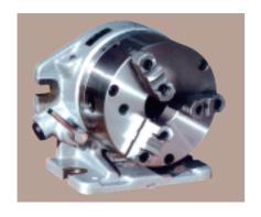
Type 1024(F2) super spacer is designed for using and indexing in both horizontal and vertical position. It is the most optimum in use for milling machines, grinding machines, drilling machines planer etc. The divisions in 2,3,4,6,8,12,24 are permitted by notched plate, any desired angular indexing can be performed too by using a graduated ring on the spindle and a verner.
