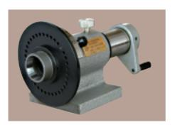
This dividing device is suitable for milling, grinding and drilling machines. It is simple in construction, easy in operation, and reliable. It not only can divide 2, 3, 4, 6, 9, 12, 18, 36 divisions, but also utilize the dividing plate and vernier hole on the body, the divisions from 1° to 360°which min. space 1° can be made
