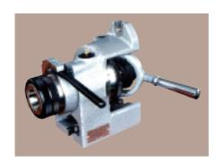
1022-0001 (FNL100B) can be mounted on milling machine, grinding machine, drilling machine and other machine tools. The divisions of 2,3,4,6,8,12, and 24 can be divided. It can also be used for marking out of components. This index has the advantage of use in horizontal and vertical, compact construction, light in weight, operating by single handle, It can accept a 5C collet. Consequently, it is a reliable device for enhancing work efficiency.
